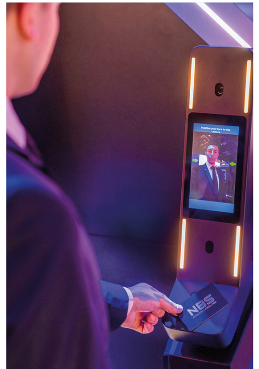
Right: NOVOVISION™ access using a player card & facial recognition to verify the card holder.
